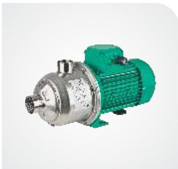
**Technical Data:****Flow:** upto 83 LPM**Head:** upto 70 m**Temp.:** -15°C to +90°CMax.**Operating Pressure:** 10 bar**Max. Inlet pressure:** 6 bar
