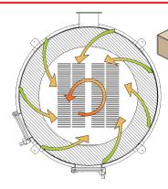
**Cycloidal air injection** leads to high residence time, less excess air and minimised combustion losses
